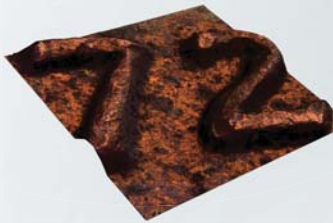
True color 3D plot of copper, showing darker blue corrosion areas
