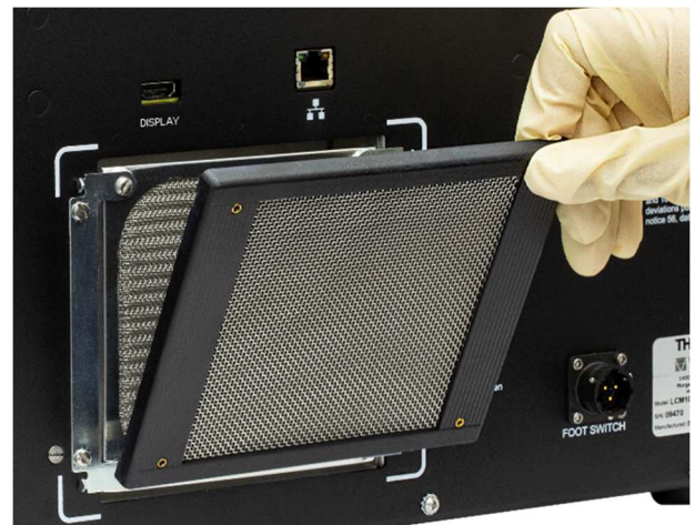
Figure 46 Removing the carbon filter cover
