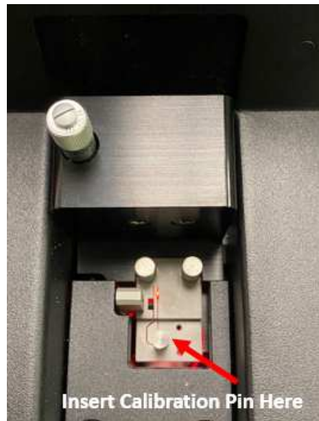
Figure 18 Inserting the Calibration Pin
