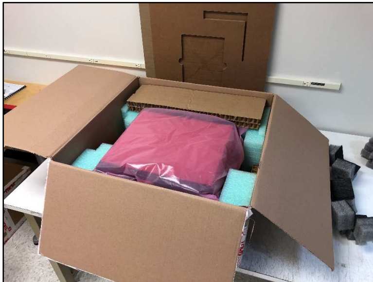
Figure 48 Addition of honeycomb spacer in inner box
