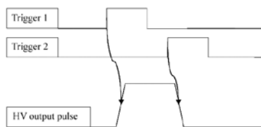
Fig. 1. Control timing charts for two-pulses controlled drivers
