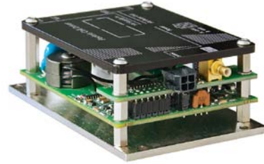
OEM version of DPS/DPD series driver with conductive pad. Suitable for repetition rate up to 50 kHz
