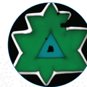
Ultra Low Frequency Raman and Photoluminescence Image of a \text{WSe}_2\text{-WSSe-WS}_2 heterojunction structure
