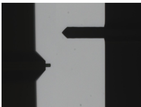
Comparison of a small and a conventional AFM cantilever. The small and regular cantilevers have tip view dimensions of 10\ \mu\text{m} \times 20\ \mu\text{m} (w x l) and 27\ \mu\text{m} \times 150\ \mu\text{m} (w x l), respectively.
