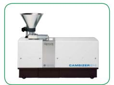
The CAMSIZER X2 has been developed to exploit dual camera technology for the measurement of fine, agglomerating powders (0.8 µm to 8 mm). To achieve accurate results for different materials, the CAMSIZER X2 offers three particle dispersion options: X-Fall for free fall dispersion (similar to the CAMSIZER P4), X-Jet for air pressure dispersion, and X-Flow for liquid dispersion.
