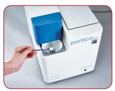
The compact Partica LA-350 laser diffraction analyzer is your routine analysis tool. It can achieve high performance with easy operation and maintenance, excelling at applications as diverse as slurries, minerals, and paper chemistry. It is the ideal combination of performance, price, and packaging to streamline particle size analysis.
