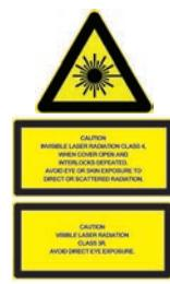
Coherent-Rofin industrial lasers are designed in strict accordance with the respective safety regulations. We certify that each laser manufactured by our company complies with FDA Radiation Performance Standards, 21 CFR Subchapter J and with IEC 60825. Warning labels as shown in the figure appear on each Coherent-Rofin laser to indicate the respective classification.
