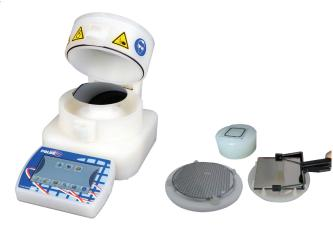
POLOS SPIN150i the best laboratory spin coater you can buy! The SPIN150i for up to 150 mm substrates includes a vacuum chuck A-V36 and fragment adapter D-V10. A variety of nozzles, megasonic cleaning and dispense lines can be added as options. The low-cost SPIN150i spin coater is suitable for processing fragments as small as 5 mm up to Ø150 mm (or 6") or 4" x 4" substrates.
