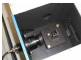
Fluorolog-QM-Trans absorbance transmission accessory
