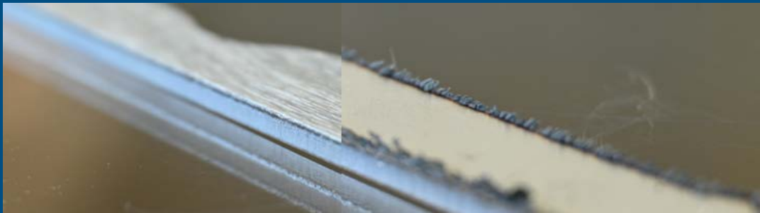
Laser cut part after and before processing with the EdgeBreaker® 6000.
