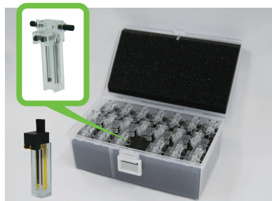
Two kind of zeta potential measurement cells (For zeta potential and particle size measurement, 100 μL, Aqueous sample and Organic solvent)
