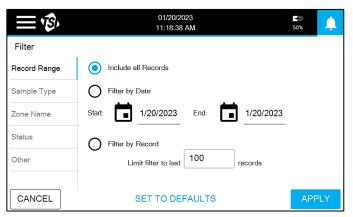
The Filter page has five screens of filtering options: Record Range, Sample Type, Zone Name, Status, and Other. Press on the tabs on the left to go to the different screens. To apply the filter(s), press the **APPLY** button.
