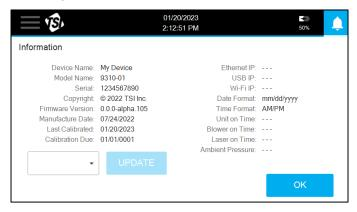
Firmware updates can be performed by inserting a USB drive with updated version of the firmware into the USB port. The list of available versions will appear in the drop-down. Select the desired version and press the **UPDATE** button. Firmware is downloaded from the TSI<sup>®</sup> website.
