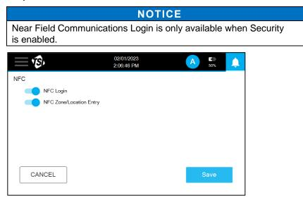
With NFC Zone/Location Entry turned on, an NFC card can be programmed by going the Sample screen in either Monitor or Classify mode. Select a Zone and Location and tap the [] icon. A prompt will appear.
