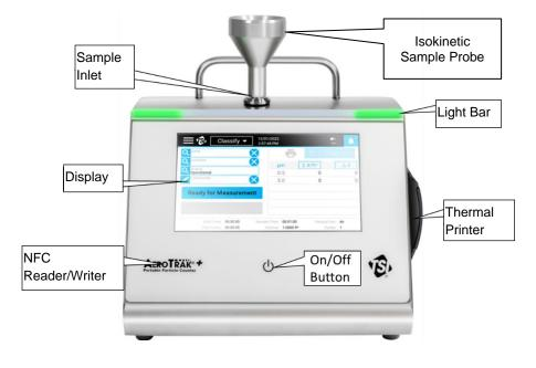
The touch-screen display provides an intuitive graphical user interface (GUI). An LED lightbar indicates when the instrument is on and provides status information during sampling. On the left side of the panel, under the AeroTrak<sup>™</sup>+ Portable Particle Counter label, is the Near-Field Communication (NFC) reader/writer that provides contactless communication.
