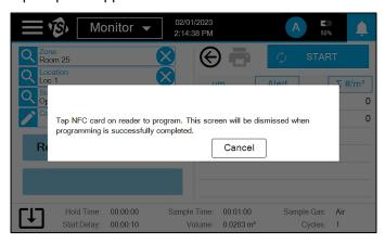
Hold an NFC card near the NFC Reader/Writer. The prompt will be dismissed and a beep will sound to indicate the card has been programmed.
