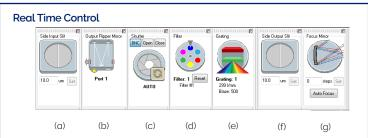
(a and f) Slit drive: Control the spectrograph slit width - drag blades on icon or type in required slit width
