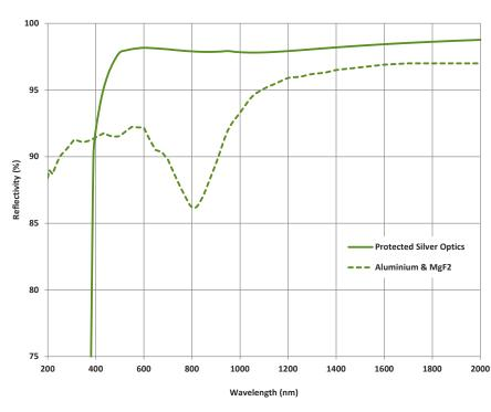
Standard systems use Al + MgF<sub>2</sub> coated optics. Protected silver optics are also available on request for maximum efficiency in the NIR region - recommended for working with Andor iDus InGaAs detectors or IR single-point detectors, such as MCT, PbS and InSb.
