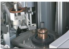
Two rotating brushes clean the upper and lower electrodes after each measurement.
