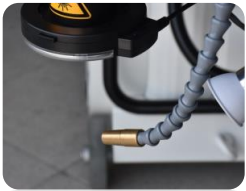
Gas feeding nozzle and acrobat light source
