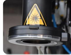
Ringlight for illumination of welding area
